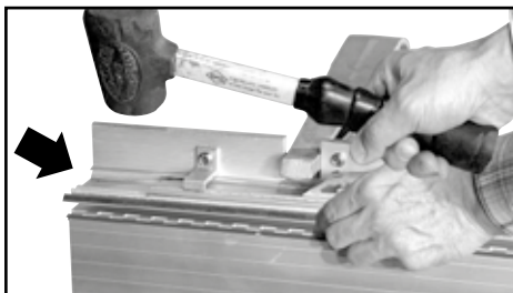
4 Install New Stainless Edge Starting on end away from Locking Handle align new Stainless Edge flush with end of Clamping Bar and tap into place sideways with Rubber Mallet.
