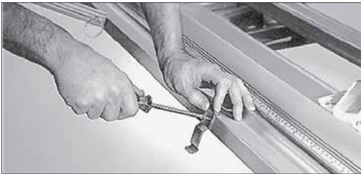
Figure 1. The Hinge Clip keeps the Moving Hinge in a 90° position for ease of aligning and cutting material. To install Hinge Clip, locate pre-drilled hole on BOTTOM right side of Moving Hinge. Align holes in Clip and Hinge as shown and insert Phillips head screw provided.
